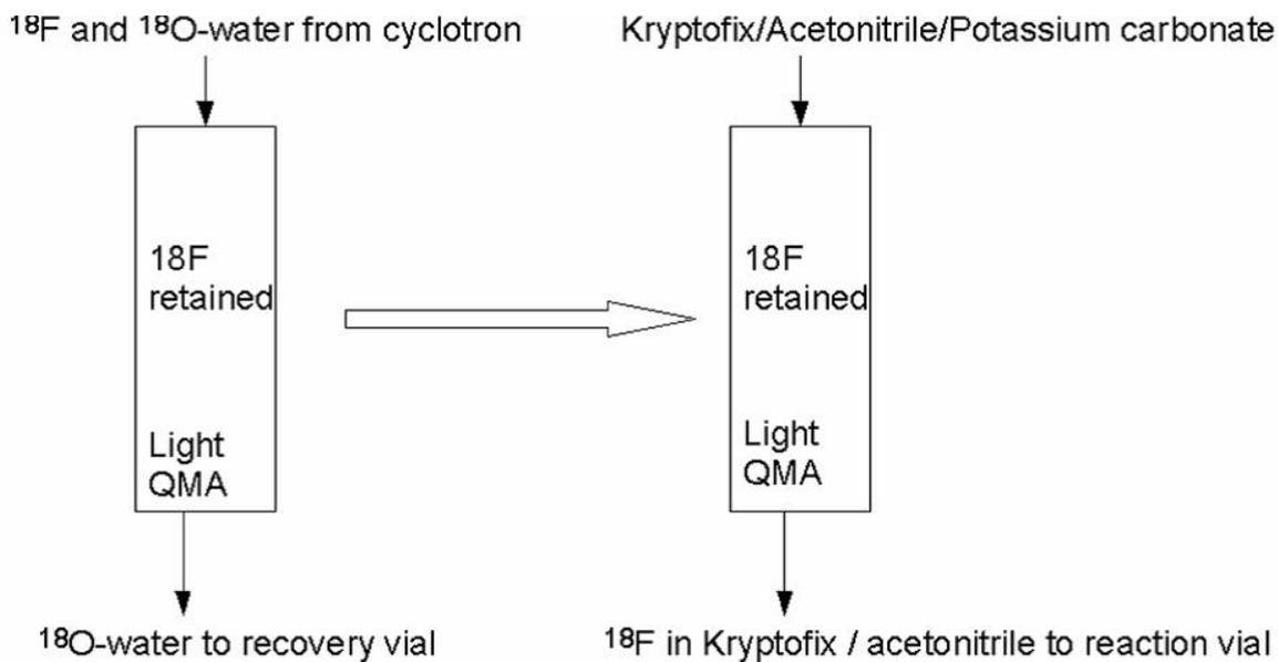
Figure (3) (a) Retention of  $^{18}\text{F}$ -FDG in light QMA ion exchange column; (b) elution of  $^{18}\text{F}$  from light QMA ion exchange column.
