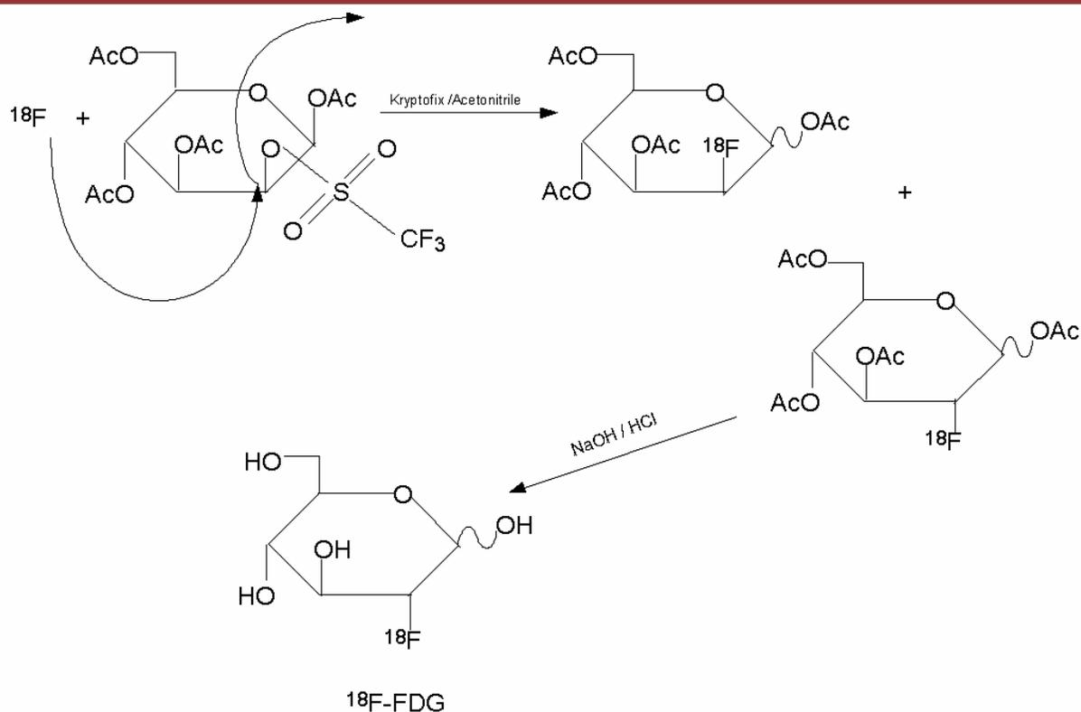
Figure (2) Synthesis of 18F-FDG by nucleophilic substitution.
